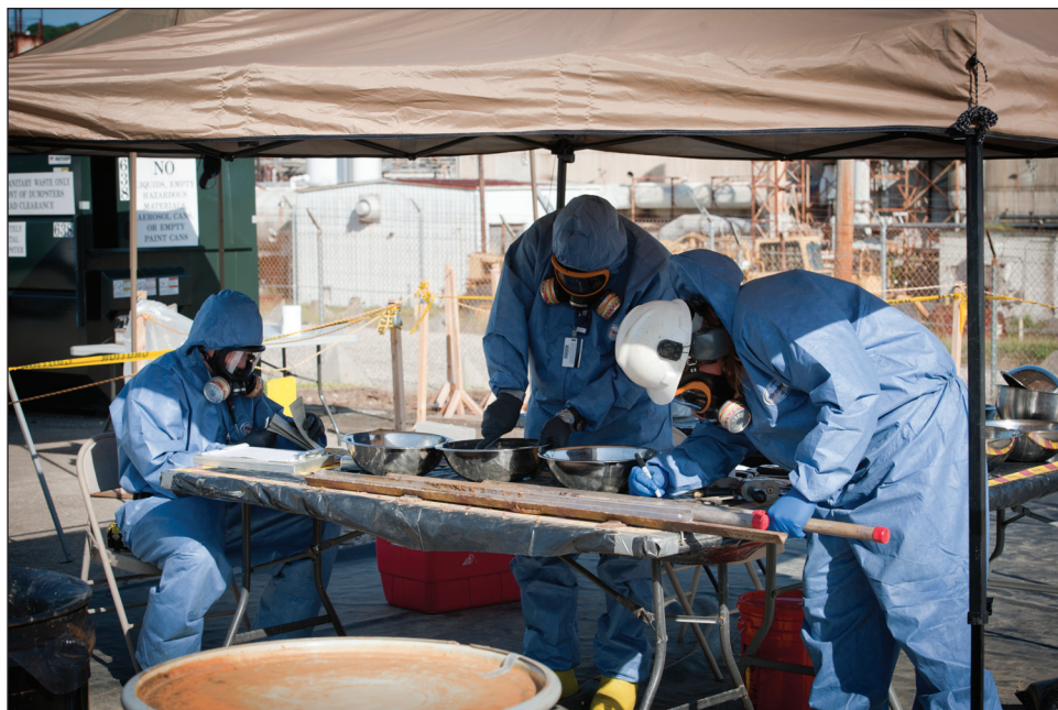
Workers prepare a soil sample for containerization at Exposure Unit 9
